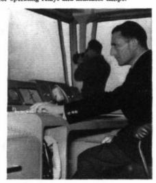
On either side of the control desk is mounted a remote indicator presenting the controller with a sensed bearing, the two units giving different bearings on different frequencies. They are fed by the Marconi AD.200 V.H.F./D.F. sets, the remote-control consoles of which are illustrated on the right.
