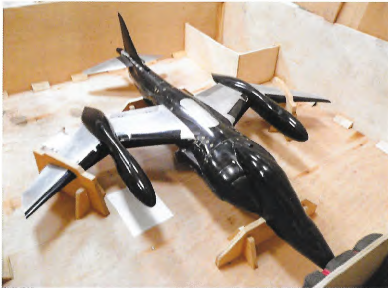
Wind tunnel model of BAe Harrier fitted with an "W" wing and tested at Farnborough
