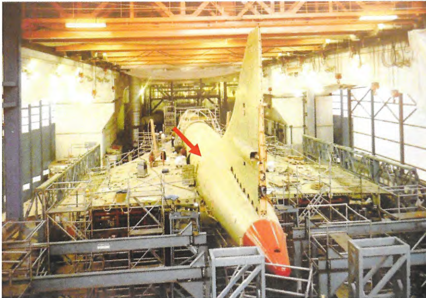
Concorde airframe 006 in the RAE Structures test rig (The FAST Concorde fuselage section (arrowed) was part of this airframe)
