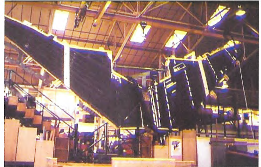
Use of carbon fibre in the construction of experimental wings for a Jaguar aircraft
